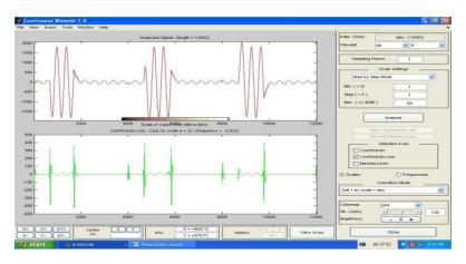
Fig8. Current response for LLLg fault at 2km by wavelet Db4
