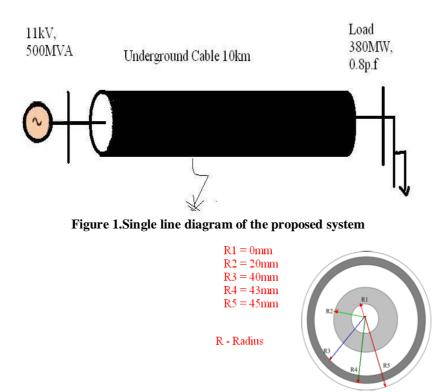
Figure2. Configuration of underground cable
