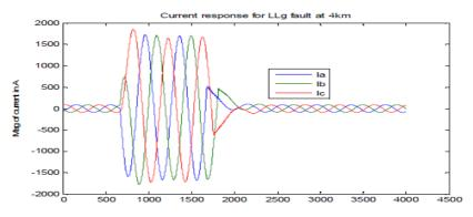
Fig 13. Current response for LLLg fault at 4km
