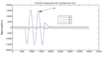
Fig 9. Current response for Lg fault at 4km
