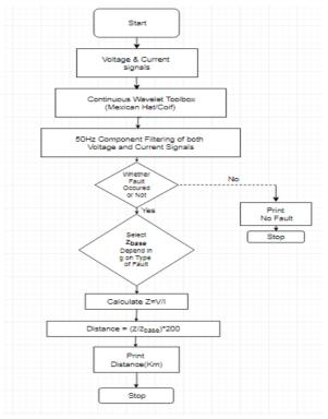
Fig.2a.The overall flowchart of the proposed algorithm
