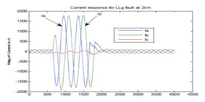
Fig5. Current response for LLg fault at 2km
