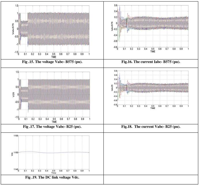
The fuzzy logic controller is found to enhance the performance of DFIG based wind farm. The dc voltage is enhance the performance comparing by conventional PI controller. The response is fast with minimum overshoots. Moreover, the steady state error after the clearance of fault is rigorously reduced
