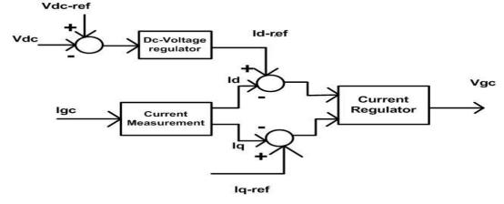
Fig .5. grid side converter control.
