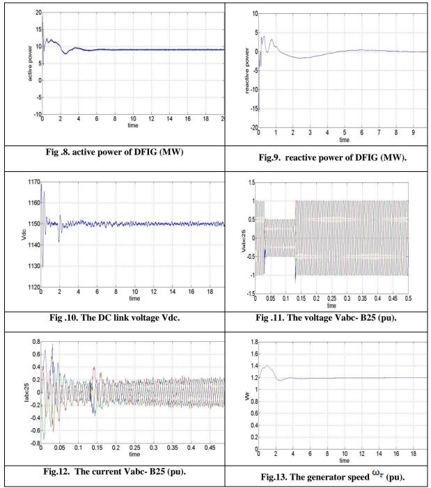
The result show the performance of the DFIG as the voltage and current after the DFIG and the voltage and current at bus 25kv. The voltage is stable at (1pu).the result also show the active power of the wind farm(9MW).and reactive power of the DFIG (0MVAR). the result also show the DFIG speed (1.2pu) and the dc voltage (1150v).
