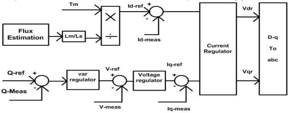
Fig .4. rotor side converter control.
