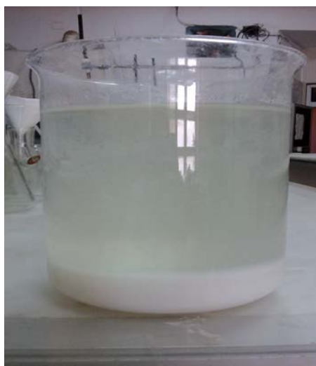
Fig. 4: Lanthanum separation (concentration) by air-ammonia method.
