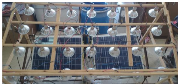
Fig 2. The PV system with the solar simulator
