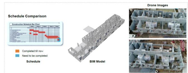
Fig. 8. The placement of windows is delayed by schedule[21].
