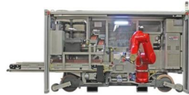
Fig. 10. The SAM100 bricklaying robot[11].
