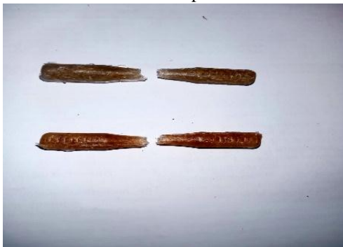
Figure 6. Common failure modes for tensile test specimens
