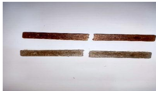
Figure 7. Common failure modes for impact specimen.
