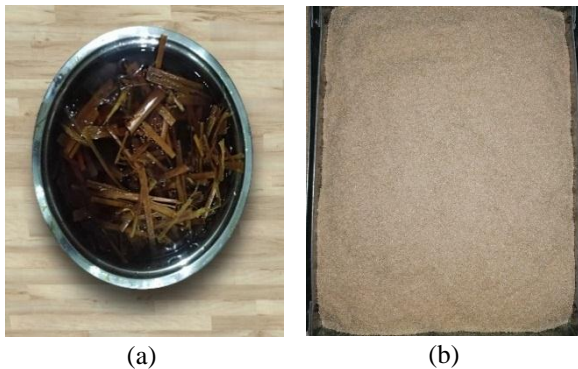
Figure 1. sugarcane bagasse fibers. (a) SCB soaked in NaOH (b) treated SCB
