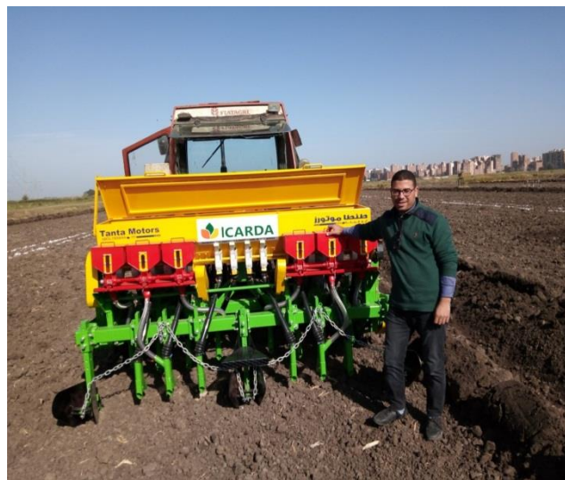
Figure 1: The Raised bed planter machine that had been used in this experiment to prepare soil for raised beds planting (from ICARDA project)
