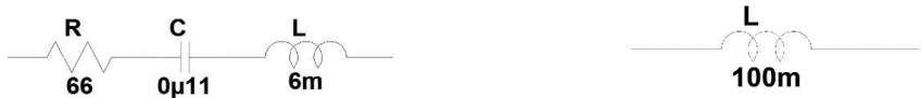
(a) Series Circuit Filter (b) Series Circuit Inductance Figure 7: Series Circuit Filterin
