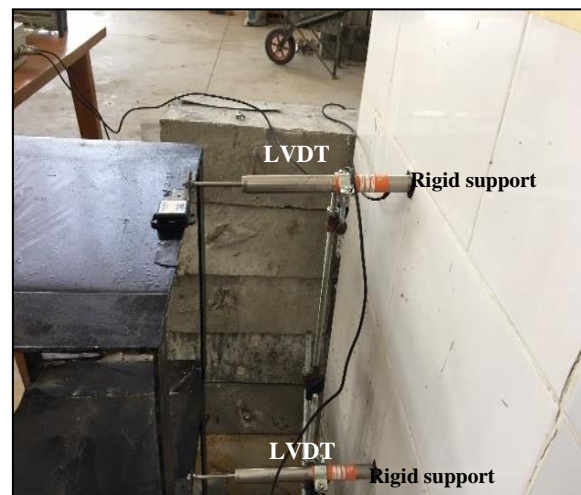
Figure 3 LVDT and Accelerometer setup.
