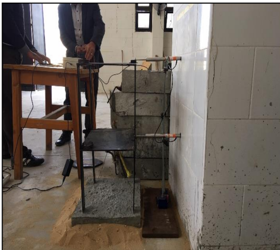
Figure 5 LVDT's connection to the model and fixation to the wall.
