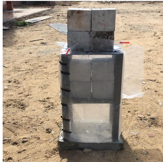
Figure 26 Laboratory model setup during ambient vibration experiment.
