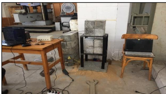
Figure 8 Test setup for the first trial with additional weight of 32 kg.
