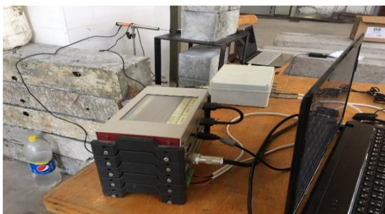
Figure 6 The connection between the LVDT - DAQ setup and the computer.
