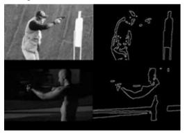
Fig 4 Segmentation by thresholding. On the left, an original image
