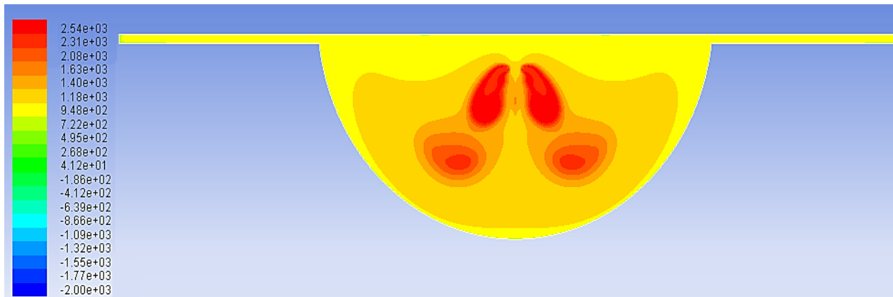
Figure 4- In-Cylinder temperature contours at 367 CA and 100% rated load
