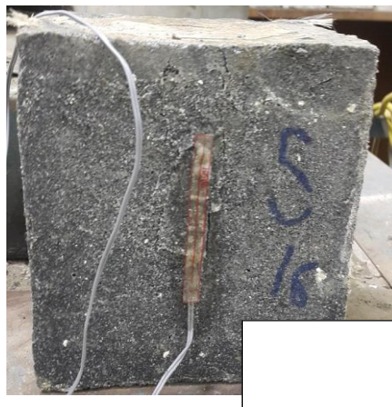
Fig.14. Compressive failure mode of specimen S16
