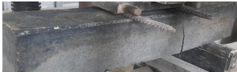
Fig.26. Failure mode of specimen S16
