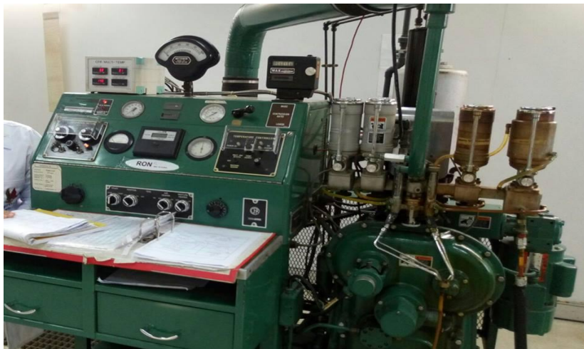
Fig (2): structure of C.F.R. used in experiments
