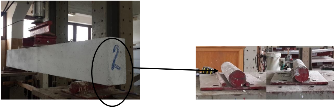
Photo (3.1): A beam specimen leveled and aligned in test setup and Details of the end supports
