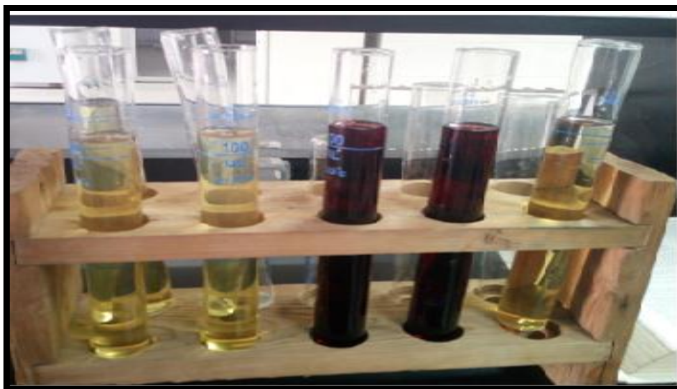
Fig. (4): The experiment of phenols ( C_6H_5OH (nm) ) in the filtered water after using the sterilized rise straw filter with sand.
