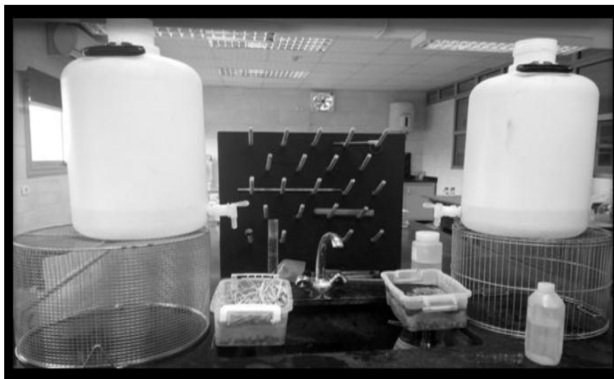
Fig. (3): The filtration process through the activated carbon with sand and sterilized rice straw with sand during autumn season
