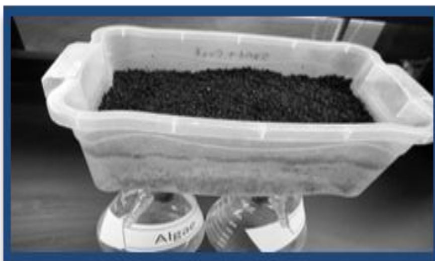
Fig. (1): Activated carbon filter with sand
