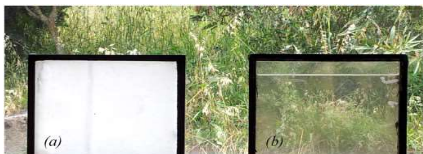
Figure 4 : PCM in solid state (a) and liquid state (b) (source : (Goia, 2017))
