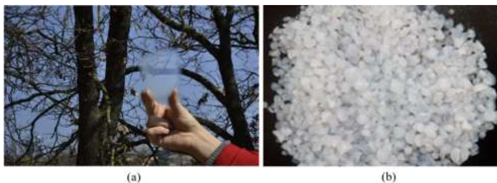
Figure 3 : a) monolithic aerogel b) granular aerogel
