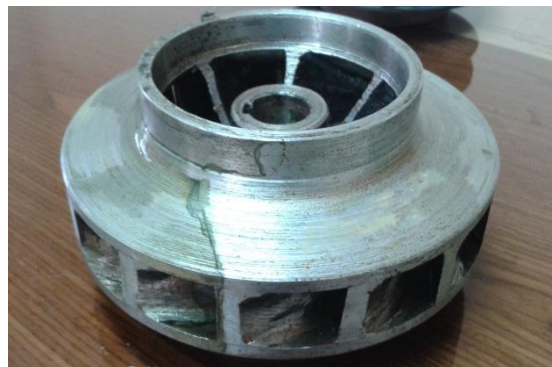
(b) Modified impeller with 7 short blades, L_b=0.25
