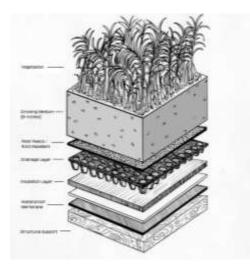
Figure 2.2 Typical green roof layers.
