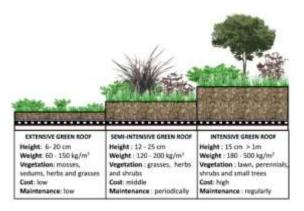
Figure 2.4 Comparison between Intensive, Semi-Intensive and Extensive Green Roofs.
