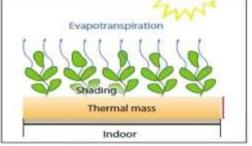
Figure 2.1 Evapotranspiration and Shading on a Green Roof.
