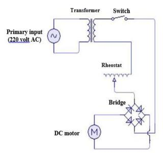
Fig. 5. Power circuit of agitator.
