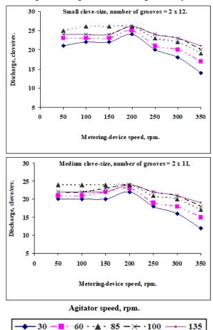
Fig. 7. Effect of metering-device and agitator speeds on garlic-cloves discharge for small and medium clove-sizes.
