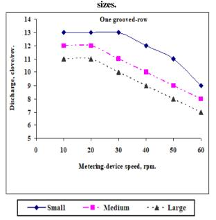
Fig. 9. Effect of metering-device and groove size on garlic-cloves discharge for one grooved-row metering device.
