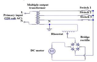
Fig. 4. Power circuit of metering device.
