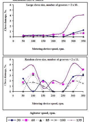
Fig. 11. Effect of metering-device and agitator speeds on garlic-cloves damage percent for large and random clove-sizes.
