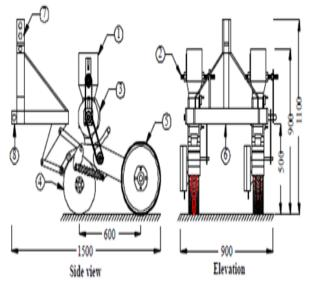
Fig. 6. Elevation and side views of the two-units garlic cloves planter.
