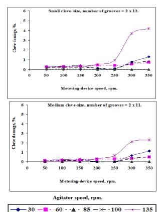
Fig. 10. Effect of metering-device and agitator speeds on garlic-cloves damage percent for small and medium clove-sizes.
