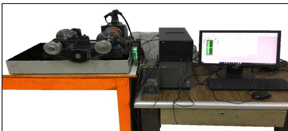
Figure 2: Configuration of data collection system.
