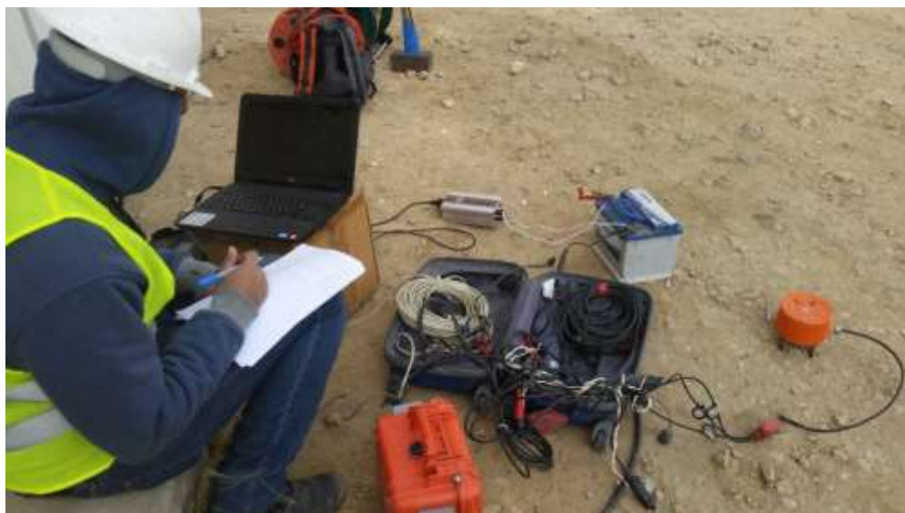
Figure 1: ES-3000 seismograph, Geometrics, USA and Traxial geophone 4.5 HZ used to determine soil amplification at Rivera City.
