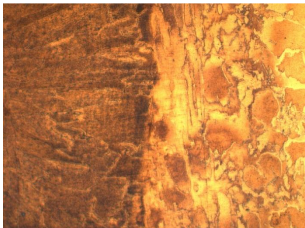
Figure 9- 1.4462 Laser weld around the weld line
