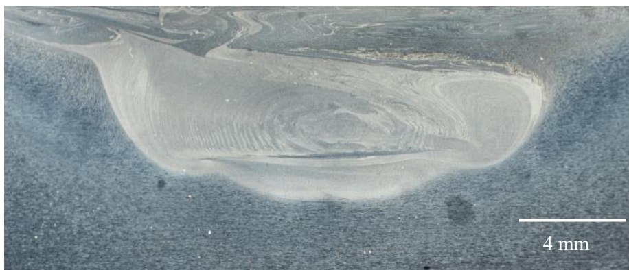
Figure 4 Macrograph of FSP stirring zone etched by Keller reagent
