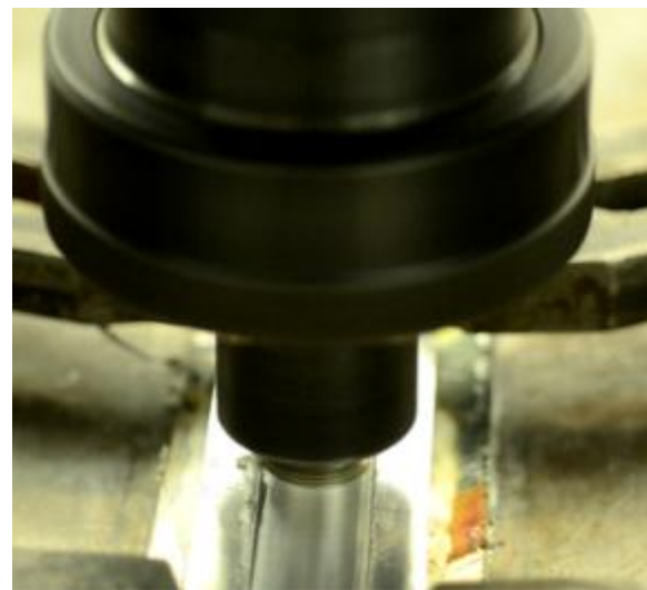
Figure 2. Friction stir welding machine spindle
