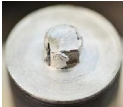
Figure 9 Aluminum deposition on square shape pin
