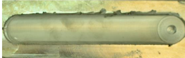
Figure 3 FSP pass with no flash and smooth surface finish
