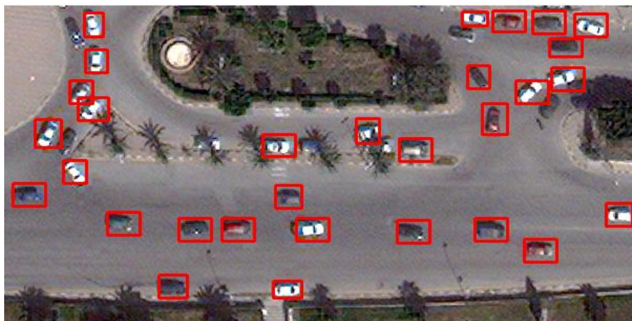
Figure 4. Vehicle detection by SSD
