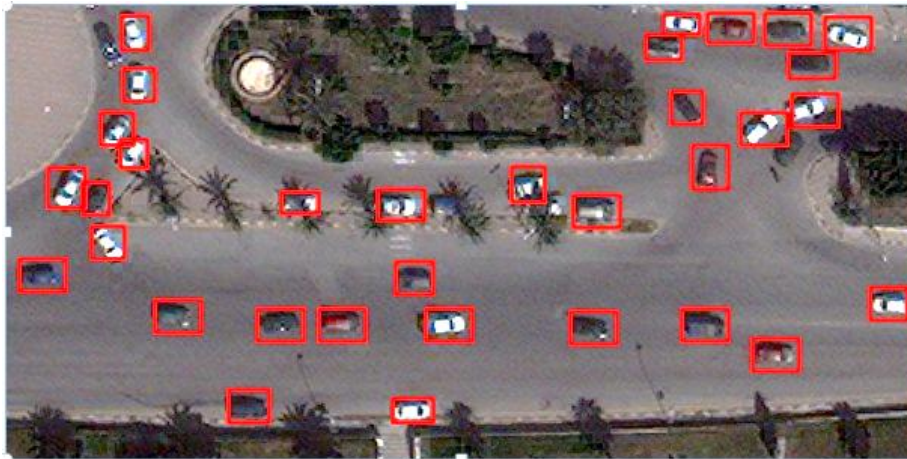
Figure 3. Vehicle detection by Faster R-CNN
