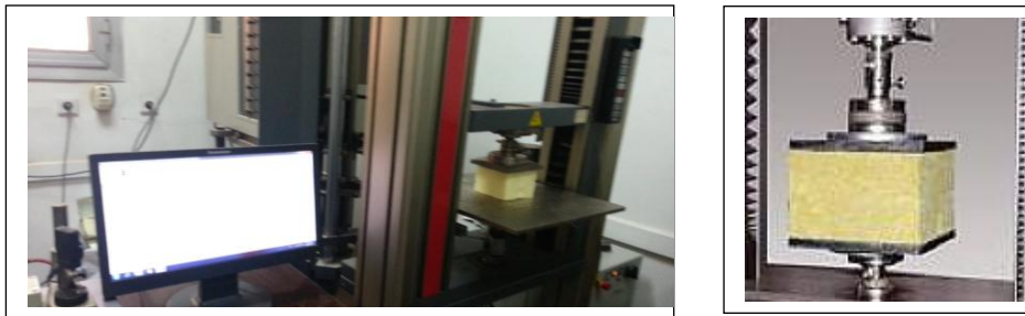
Figure 6: Zwick Roell device (Germany), compressive strength determination
