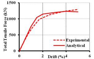
Figure 8: Comparison Between analytical and experimental results for Tensile Force
