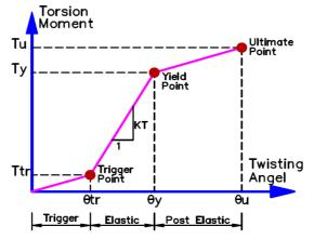
Figure 17: Typical torsion – twisting angle envelope curve of the hysteretic cyclic torsion response
