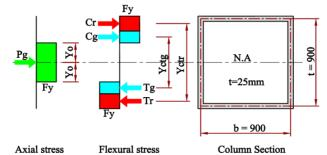
Figure 11: Plastic stresses distribution on column box section
