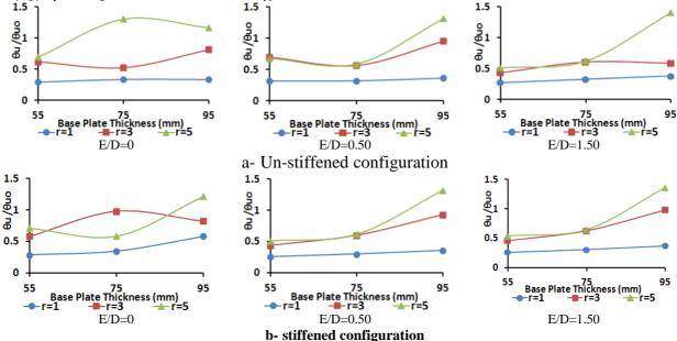
Figure 16: Relative ultimate twisting angle variation with base plate thickness
