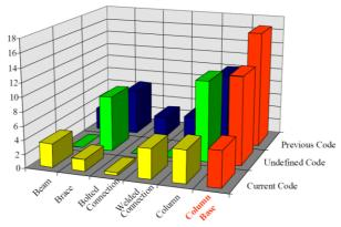
Figure 1: Statistical analysis of the structural damage compiled after the 1995 Hyogo-ken Nanbu earthquake [1].
