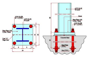
Figure 3: Details of verification model (All Dim. in inch) Table 1 Mechanical Properties of Connection Elements
