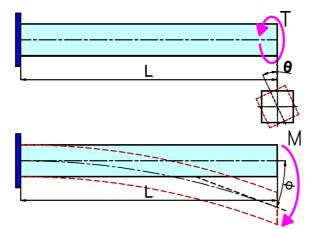
Fig. 13: Beam deformed shape under bending and twisting loading
