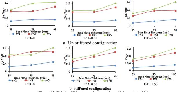
Figure 15: Relative Ultimate torsion variation with base plate thickness
