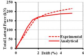
Figure 7: Comparison Between analytical and experimental results for Lateral Force
