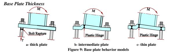
As per literature Behavior of base connection is sensitive to the base plate thickness. As illustrated in Figure 9 the Behavior of base plate is classified for 3 classes according to the expected mode of failure; thick plate behavior, intermediate plate behavior, and thin plate behavior. In this study three parametric values has been adopted to capture as much as possible the expected modes of failure previously mentioned, the selected values shall be 55mm, 75mm, and 95mm.
