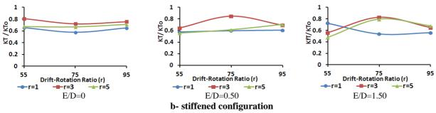
Figure 19: Typical Relative torsional stiffness variation with base plate thickness
