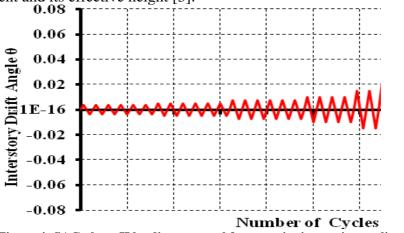
Figure 4: SAC phase II loading protocol for stepwise increasing cyclic test[3]
