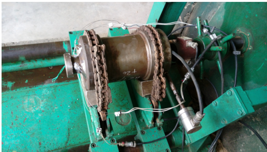
Figure 1 Photo of the 6 inch motor on the test stand.
