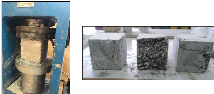
Fig. 4. Compressive Strength Test.
