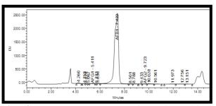
Fig. (8): HPLC chromatogram of AFs in positive sample of peanut from Faraskour region.
