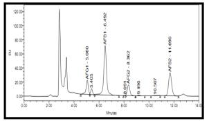
Fig. (5a): HPLC chromatogram standard of AFs.
