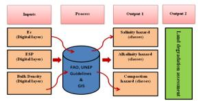
Fig. 3: Simple Cartographic Model used to assess the Land Degradation Hazard
