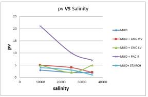
Fig. 2: Salinity concentration vs. PV for four types of polymers.
