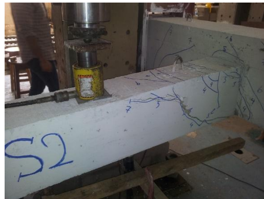
Fig. 11: Specimen-S2 crack pattern at failure
