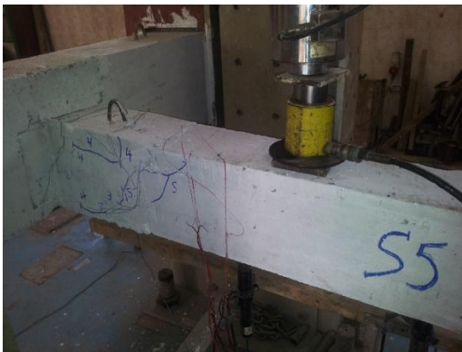
Fig. 14: Specimen-S5 crack pattern at failure
