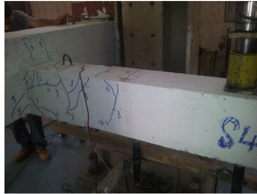
Fig. 13: Specimen-S4 crack pattern at failure
