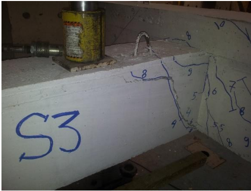
Fig. 12: Specimen-S3 crack pattern at failure
