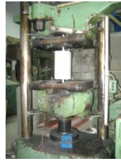
Fig. 7: Test setup for direct tension test.
