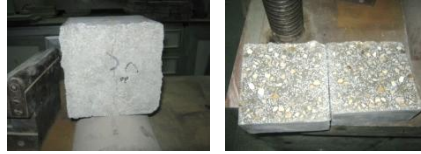
Fig. 15: Failure pattern of FBLWC cube specimens
