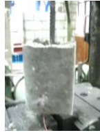
Fig. 18: Lateral cracks due to direct tension test for FBLWC
