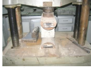
Fig. 6: Splitting tensile test on concrete cube specimens
