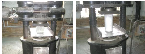
Fig. 2: Cylinder and cube specimens in the compression machine.
