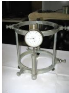
Fig. 3: The test cylinder fitted with the compressometer
