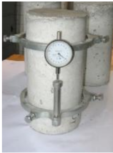
Fig. 3: The test cylinder fitted with the compressometer
