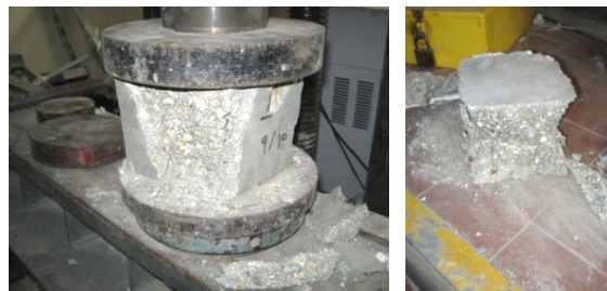
Fig.13: Failure stages during the UTM machine for C6
