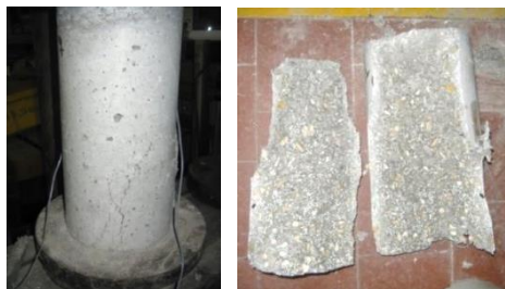
Fig. 14: Failure stages during the UTM machine for CY7
