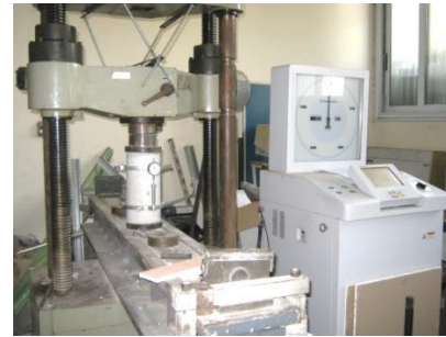
Fig. 4: Specimen's setup for E-modulus test
