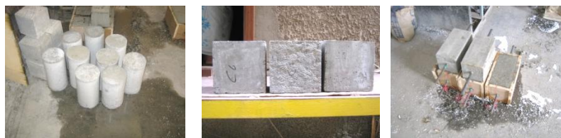
Fig. 1: cube, cylinder and prism specimens after being removed from the molds and curing
