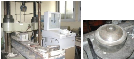
Fig. 5: (A): Test setup of cube specimens for the determination of the stress-strain relationship, (B) Poll seating
