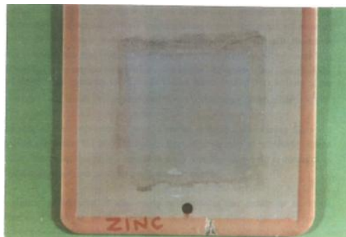
Plate.6: ZE sample after 337hrs of immersion in 3 %NaCl
