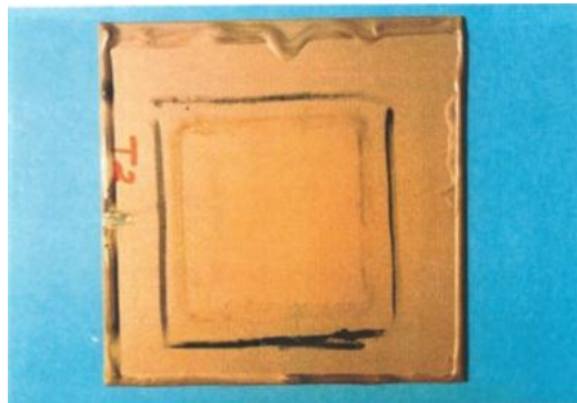
Plate.4: SIL after 204 hrs of immersion in 3 %NaCl
