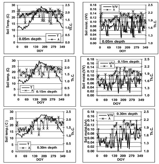
Fig. (3): Thermal conductivity (Th.C.) affected by soil temperature (°C) and soil moisture content (m<sup>3</sup>/m<sup>3</sup>) through 51 observations at three depths (DOY=Day Of Year).
