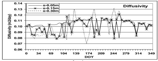
Fig. (6): Soil thermal diffusivity (m<sup>2</sup>day<sup>-1</sup>) for three depths at 51 observation for three soil depths (DOY = Day Of Year).
