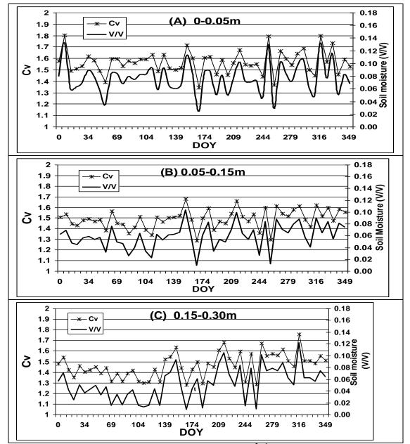
Fig.(1):Soil volumetric heat capacity (CV) (MJm<sup>-3</sup>c<sup>-1</sup>) and volumetric moisture content (v/v) (m<sup>3</sup>m<sup>-3</sup>) of the three soil depths (A,B and C), (DOY=Day of Year).
