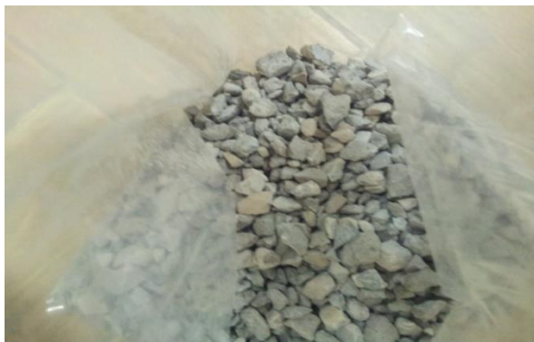
Figure (2): Demolition waste after mechanical preparation
