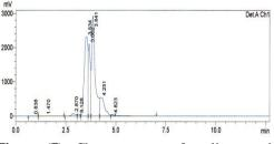
**Figure (7):** Chromatogram of proline standard, that appeared at 3.84 minutes by use 40 mM Na<sub>2</sub>SO<sub>4</sub> phase in HPLC technique.
