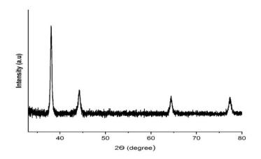
Figure (1): A typical XRD pattern of prepared AgNPs.
