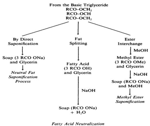
Figure 1: Three processes for making soap from triglycerides [5]
