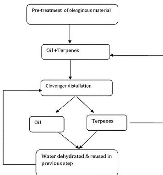
**Figure 3: Block flow diagram of green solvent technology [23]**
