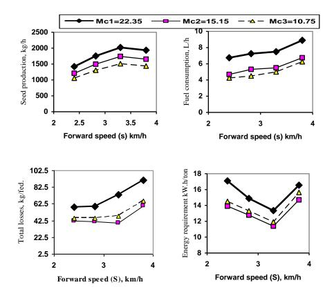
Figure 3. Effect of both forward speed and seed moisture content on seed production (kg/h), total loss kg/fed, fuel consumption (L/h), and specific energy requirements (kW.h/ton).
