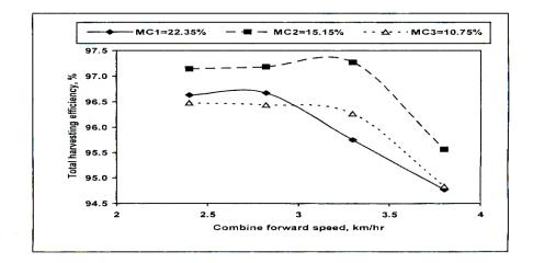
Figure 4. Effect of combine harvester forward speed and seed moisture contents on total harvesting efficiency, %.
