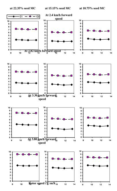
Figure 1. Effect of rotor speed and rotor-concave clearance ratio on total losses, at different forward speed and seed moisture contents
