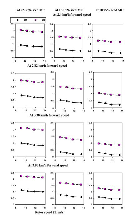
Figure 5. Effect of rotor speed and rotor-concave clearance on separating losses, at different forward speeds and seed moisture contents ( $c_1 = 1.5:1, c_2=1.3:1$ ).
