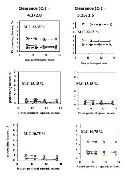
Figure 7. Effect of threshing rotor peripheral speed and rotor-concave clearance ratio on processing losses at different of seed moisture content.
