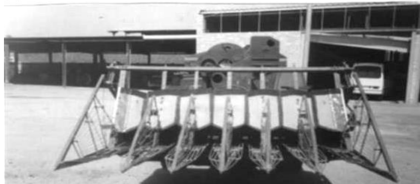
Figure (2): The modified header, a, under the platform b, under the platform
