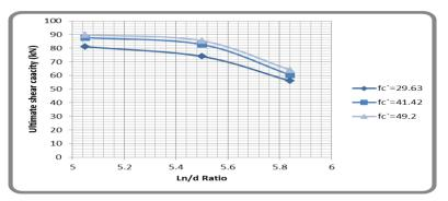
Fig. (20) Effect of clear span to the effective depth ratio (ln/d) on the ultimate shear strength for I- section.
