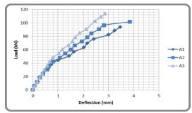
Fig. (6): Load –deflection curve for SCC rectangular beams at compressive strength  $(f_c^{'})$  =29.36 Mpa.
