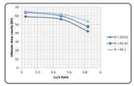
Fig. (19): Effect of clear span to the effective depth ratio  $(\ln/d)$  on the ultimate shear strength for T- section.
