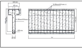
Fig. (2): Details of T-section all dimensions in mm.
