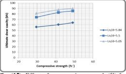
**Fig. (15):** Effect of compressive strength  $(f'_c)$  for SCC rectangular beams on the ultimate strength.
