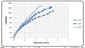
Fig. (11): Load –deflection curve for SCC T-section beams at compressive strength  $(f_c') = 49.2$  Mpa.
