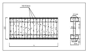
Fig. (3): Details of I-section all dimensions in mm.
