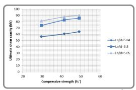
**Fig. (17):** Effect of compressive strength  $(f_c)$  for SCC I-section beams on the ultimate strength.
