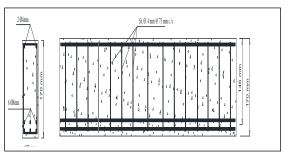
**Fig. (1):** Details of rectangular section all dimensions in mm.
