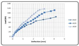
**Fig. (9)** Load –deflection curve for SCC T-section beams at compressive strength  $(f_c') = 29.36$  Mpa.
