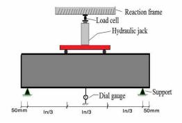
Fig. (4): Schematic diagram of test set-up.
