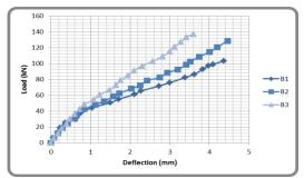
**Fig.** (7): Load –deflection curve for SCC rectangular beams at compressive strength  $(f_c)$  =41.42 Mpa.
