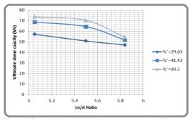
Fig. (18): Effect of clear span to the effective depth ratio  $(\ln/d)$  on the ultimate shear strength for rectangular section.
