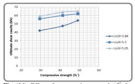
Fig. (16): Effect of compressive strength  $(f_c)$  for SCC T-section beams on the ultimate shear strength.
