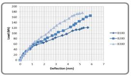
**Fig. (13):** Load –deflection curve for SCC Isection beams at compressive strength  $(f_c)$  =41.42 Mpa.
