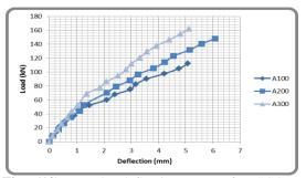
Fig. (12): Load –deflection curve for SCC Isection beams at compressive strength  $(f_c)$  =29.36 Mpa.
