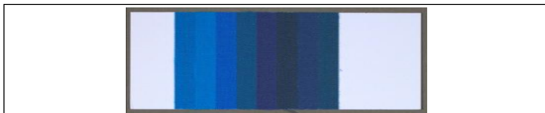
Figure 12 ISO's Blue Wool standard cards [43]. Where sample 1 is extremely sensitive to light, while sample 8 is the most stable dye [16].
