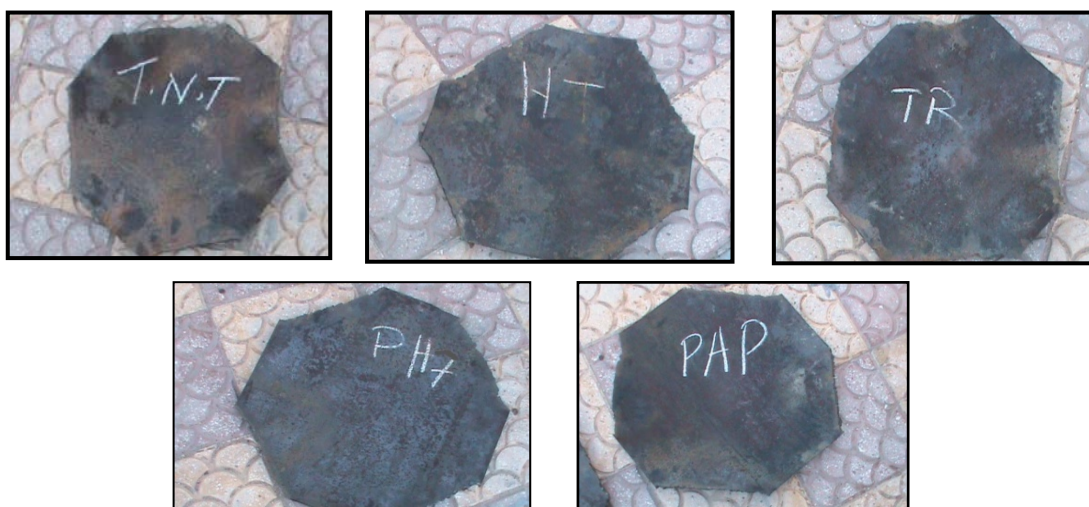
Figure 9. Plate deformation caused by underwater explosions
