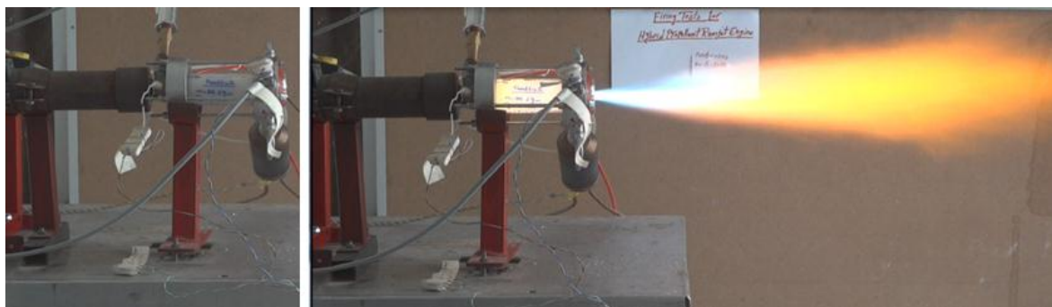
Figure 8. Tested engine mounted on test stand
