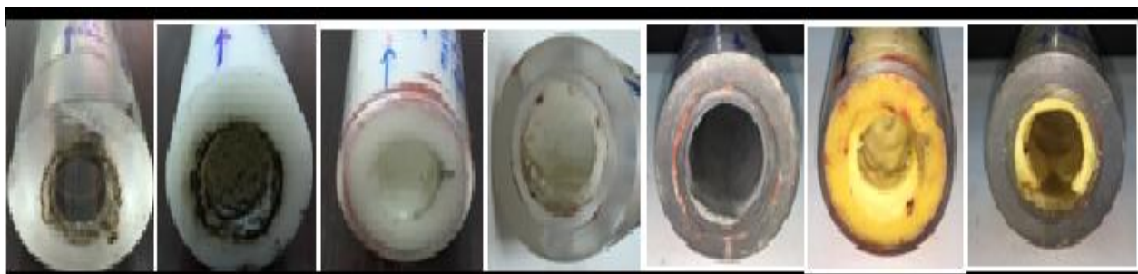
Solid fuel grain inlet port after firing
