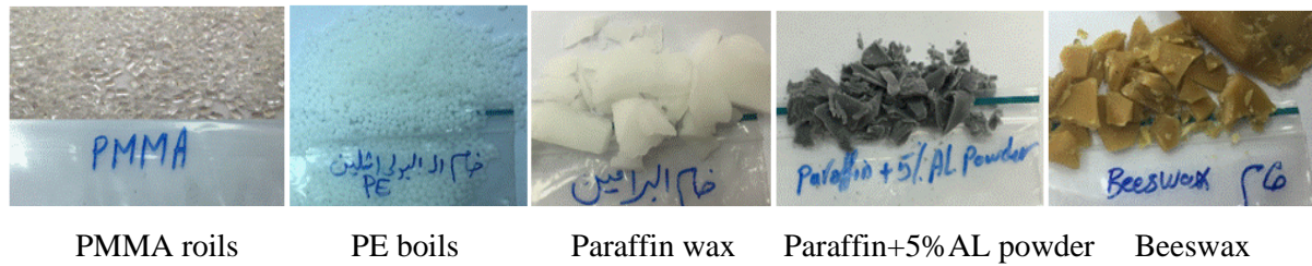
Figure 2. Solid fuel grain original role material
