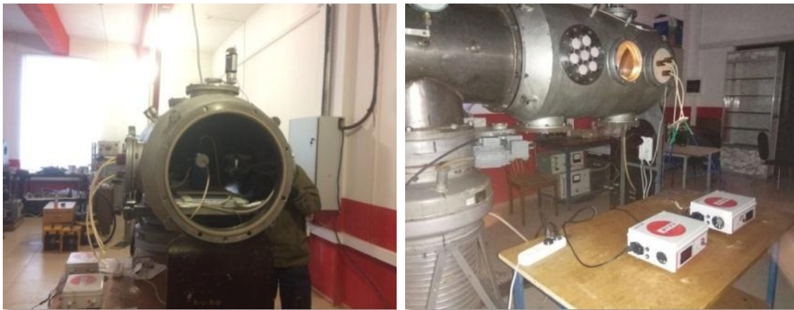
c) PPT inside vacuum chamber
