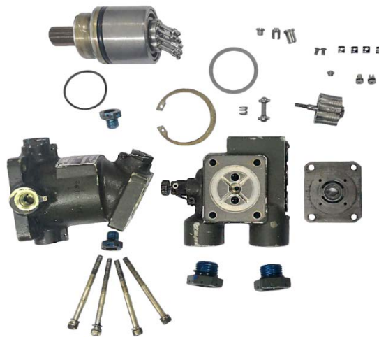
Figure 8. Disassembled hydraulic motor.
