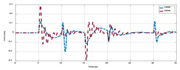
Figure 27. Pitch control for BS-PID controller tuned by LOPID and FOPID under effect of wind disturbance.
