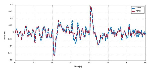
Figure 30. Roll control for BS-PID controller tuned by LOPID and FOPID under effect of noise.
