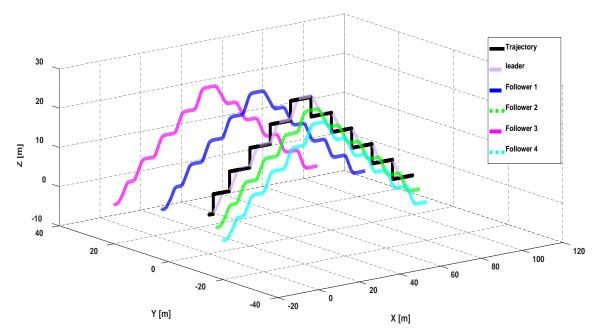
Figure 10. Trajectory tracking of BS-PID controller tuned by LOPID for cooperative quadrotors in *XYZ*-orientation.
