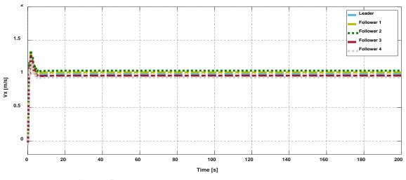
Figure 15. Velocity of cooperative quadrotors in X-orientation.
