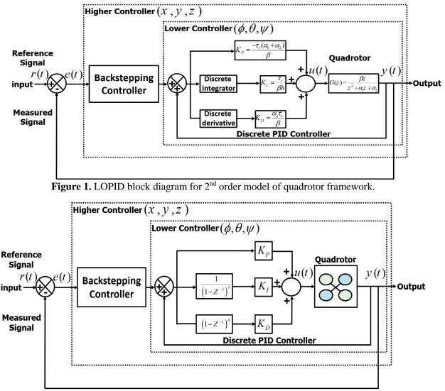
Figure 2. FOPID block diagram for 2<sup>nd</sup> order model of quadrotor framework.
