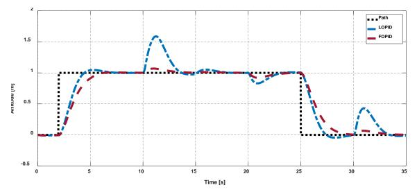
Figure 25. Trajectory tracking of BS-PID controller tuned by LOPID and FOPID for the leader of the cooperative quadrotors in Z-orientation under effect of wind disturbance.
