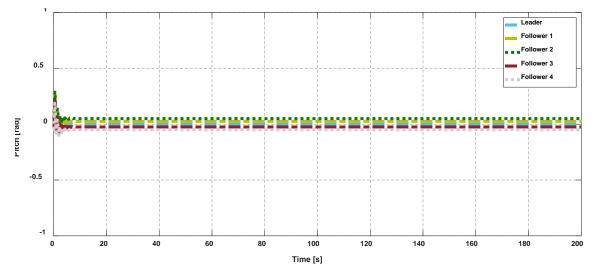
Figure 23. Pitch control of BS-PID controller tuned by FOPID for cooperative quadrotors.
