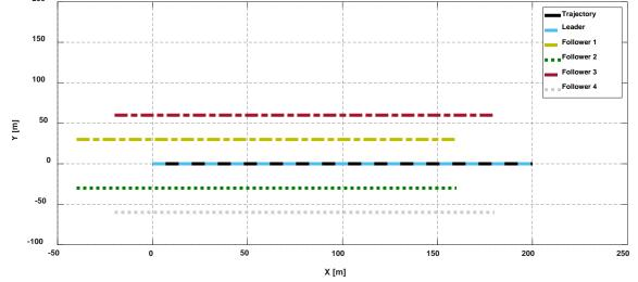
Figure 20. Trajectory tracking of BS-PID controller tuned by FOPID for cooperative quadrotors in *XY*-orientation.
