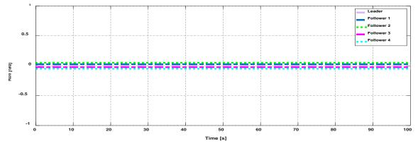
Figure 11. Roll control of BS-PID controller tuned by LOPID for cooperative quadrotors.
