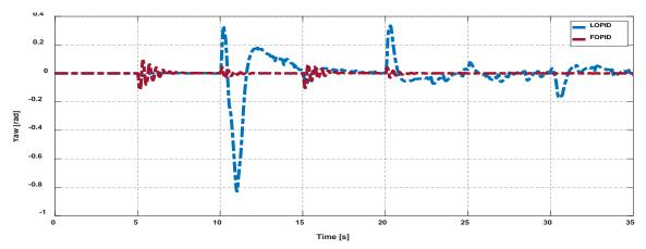
Figure 28. Yaw control for BS-PID controller tuned by LOPID and FOPID under effect of wind disturbance.
