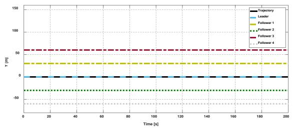
**Figure 16.** Trajectory tracking of BS-PID controller tuned by FOPID for cooperative quadrotors in *Y*-orientation.
