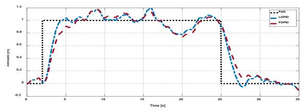
Figure 29. Trajectory tracking of BS-PID controller tuned by LOPID and FOPID for the leader of the cooperative quadrotors in Z-orientation under effect of noise.
