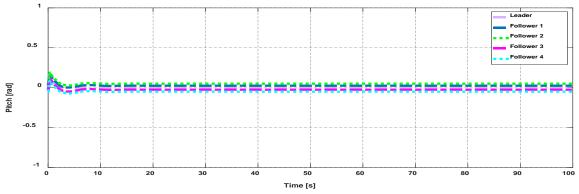
Figure 12. Pitch control of BS-PID controller tuned by LOPID for cooperative quadrotors.
