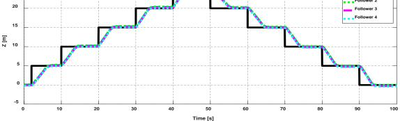
**Figure 7.** Trajectory tracking of BS-PID controller tuned by LOPID for cooperative quadrotors in **Z**-orientation.
