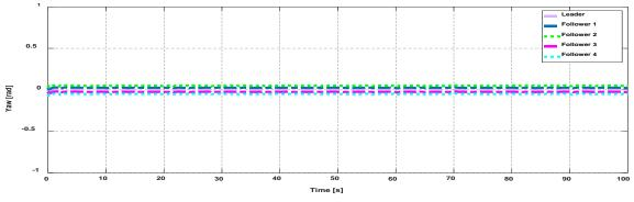
Figure 13. Yaw control of BS-PID controller tuned by LOPID for cooperative quadrotors.
