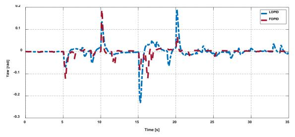
Figure 32. Yaw control for BS-PID controller tuned by LOPID and FOPID under effect of noise.
