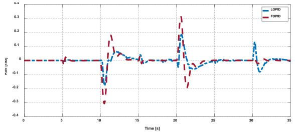
Figure 26. Roll control for BS-PID controller tuned by LOPID and FOPID under effect of wind disturbance.
