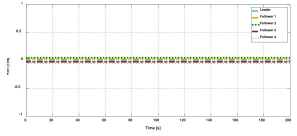
Figure 22. Roll control of BS-PID controller tuned by FOPID for cooperative quadrotors.
