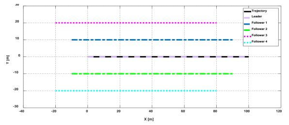
**Figure 9.** Trajectory tracking of BS-PID controller tuned by LOPID for cooperative quadrotors in *XY*-orientation.
