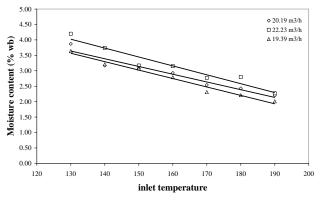
Fig. 3. Powder moisture content as a function of inlet air temperature and drying air flow rate for compressed air flow rate of 600 L/h
