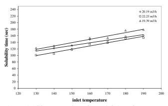
Fig. 6. Powder solubility as a function of inlet air temperature and drying air flow rate for compressed air flow rate of 800 L/h
