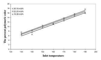
Fig. 9 the percent polymeric color as a function of inlet air temperature and drying air flow rate for compressed air flow rate of 600 L/h
