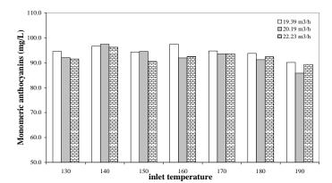
Fig. 8. Powder monomeric anthocyanins content as a function of inlet air temperature and drying air flow rate for compressed air flow rate of 800 L/h
